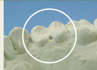
Stone model with hydrogen evolution voids
